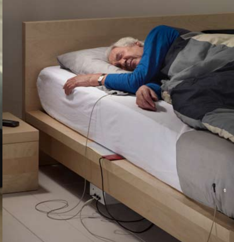
Heart rate is measured using ECG textile sensors in the pillow case and bed sheet while the patient is asleep.
